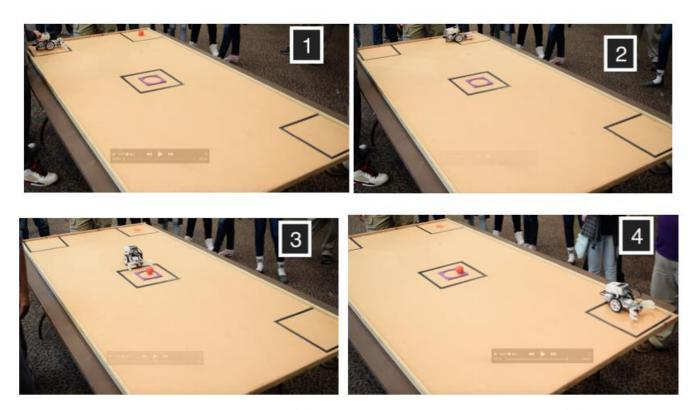
The robot will travel from the start position (1) to retrieve the ball in the top left corner (2), then deliver it to the pedestal in the middle (3). Lastly, robots park completely within the top right square after delivering the ball (4). The ball is the standard red ball from the **LEGO NXT** kits, and the holder is made from 7m straight beams and 4 L-shaped connectors.
