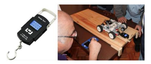
You can hook the scale to the back of the robot via the attached hook.
